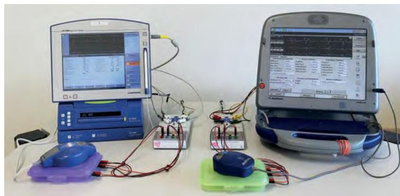
**Fig. 2:** Typical equipment of one learning station used for practical in-vitro hands-on training on 'Individual Pacemaker Setup and Measurements'. Current Pacemaker-programmers (left: Biotronik ICS 3000, right: Medtronic 2090); below: pacemakers mounted into special connection boxes with attached programming head, which is operated via a connection module of the cardiac rhythm simulators InterSim II USB (in the middle).
