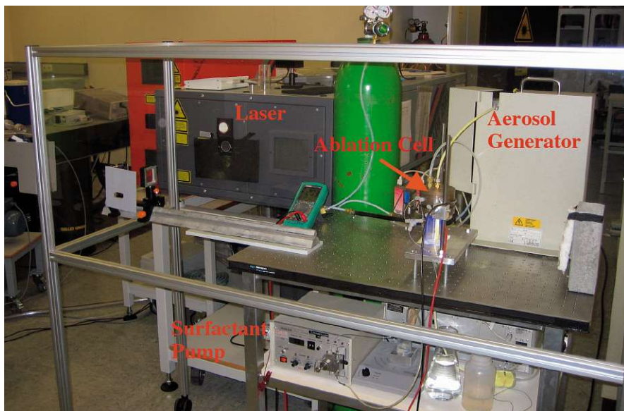
Fig. IV.6-3: LAM Setup with its main components
