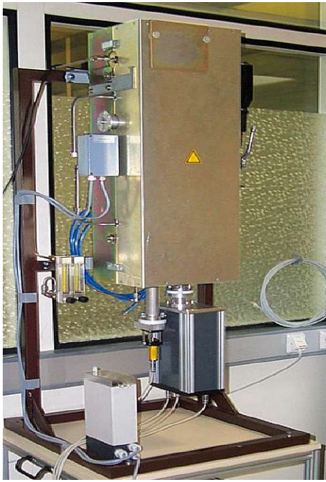
Fig. IV.4-3: Long Path Multi-wavelength Extinction LPME
